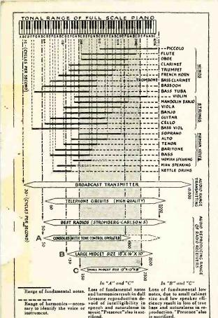
Chart prepared by the Stromberg-Carlson Acoustical Laboratories showing tonal range of the various types of receivers.
