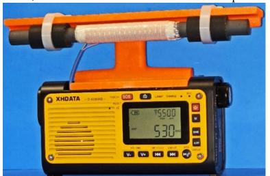
receiver with a 3000 mAh "18650" lithium battery, a built-in emergency flashlight, emergency hand crank and solar panel for charging the battery, an MP3 player with Bluetooth capability and a superb 5 watt-rated speaker (although the audio output power is only 2 watts).
