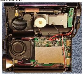
the back panel. These self-tapping screws are small, tightly installed and obviously not meant to be played with. After using a jeweler's screwdriver to remove all of them, I got the distinct impression that XHDATA would probably want to replace any defective radios rather than repair them.
