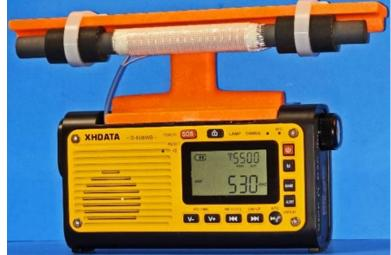
receiver with a 3000 mAh "18650" lithium battery, a built-in emergency flashlight, emergency hand crank and solar panel for charging the battery, an MP3 player with Bluetooth capability and a superb 5 watt-rated speaker (although the audio output power is only 2 watts).
