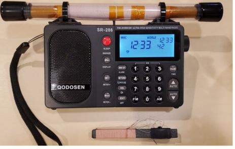
the motor do the winding. All I had to do was guide the successive turns as the rod rotated. It took only a couple of minutes to complete, and the coil turned out very neat with no gaps in the winding.
