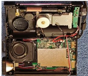
self-tapping screws are small, tightly installed and obviously not meant to be played with. After using a jeweler's screwdriver to remove all of them, I got the distinct impression that XHDATA would probably want to replace any defective radios rather than repair them.
