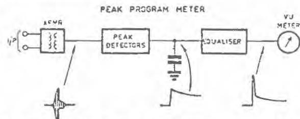
Figure 1. Block diagram of Peak Programme Meter.
