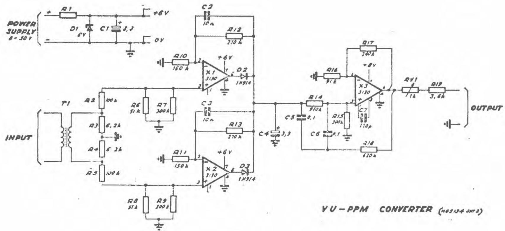
Figure 2. Circuit diagram of vu to ppm converter.
