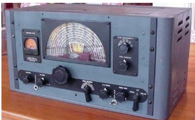
At left: an RME-45 receiver from the late 1940s. 10 tubes, covers 540 kHz to 33 MHz.
