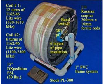
over the new 12" FSL with the 660/38 Litz wire – and very fortunately, an even greater sensitivity advantage over the 2013 DXpedition 12" model. As such, the new 1162/46 Litz wire, dual coil 12" FSL was chosen as the winning antenna for this April 9-11 DXpedition to the "Rockwork 4" ocean cliff site.
