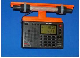
The 7.5" loopstick Tecsun PL-380 model definitely has better construction to survive heavy rain and nasty bumps, but its 1 kHz DSP filtering tends to clip off some of the higher audio frequencies during MP3 recordings. The CCrane SWP with the transplanted IF filter (an early 2009 concoction) can provide better MP3 recording audio, but any type of rain can disrupt the tuning operation of its razor-sharp Slider loopstick. As such, these two
