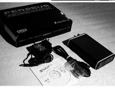
The Perseus is a direct-sampling software-defined radio (SDR) receiver offering continuous 10 kHz - 30 MHz coverage. Unit is in like-new condition, and comes complete with USB cord, AC adapter, SO239 to BNC RF adapter, software CD, and manual. More information on this receiver can be found on line at various sites, including microtelecom.it/perseus.
