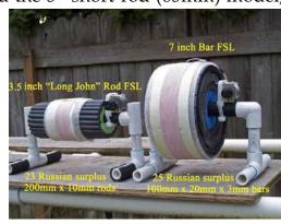
different antennas deadlocked in performance on all 5 of the test signals. This was the first weak-signal deadlock in 10 different FSL match ups, so it was quite a surprise. Both antennas were then tested against the 4' air core reference loop – and both FSL's deadlocked with it, also! There was now no doubt that the DXing performance of these two radically different models was identical, which certainly was a puzzle considering their polar-opposite design.
