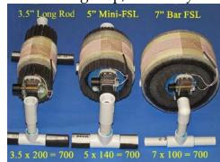
One school of thought held that coil diameter was the most important gain factor, while another was that ferrite size and weight was paramount. Ferrite rod versus ferrite bar opinions were also diverse, and even Litz wire variables became part of the controversy. Any newcomer wishing to build an FSL antenna had no shortage of advice – the only problem was which advice to follow.
