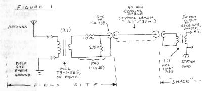
Note that the field site transformer provides broadband impedance matching (9:1 step down from approximately 450 ohms antenna to 50 ohms transmission line) as well as ground isolation. One could use either the Mini-Circuits T9-1-X65 or an equivalent homebrew model - for instance, Nick's FT50-43 Amidon core with 35 turns primary, 11 turns secondary. Other ratio transformers (e. g. 1:1, 4:1, 16:1) may be tried; in some circumstances, a different ratio might provide more signal transfer.
