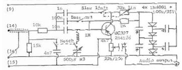
Power is derived from the 6.3Vac "Break In" relay supply (9), turn Break In "On":
